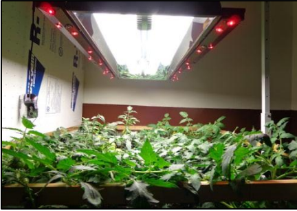
Asymmetrically placed diodes on 10° planes allow for wider flowering areas with increased canopy penetration. Here you can see the 660nm diodes running at lights on. The diodes that are not on are the 730nm diodes that only run at lights out.
